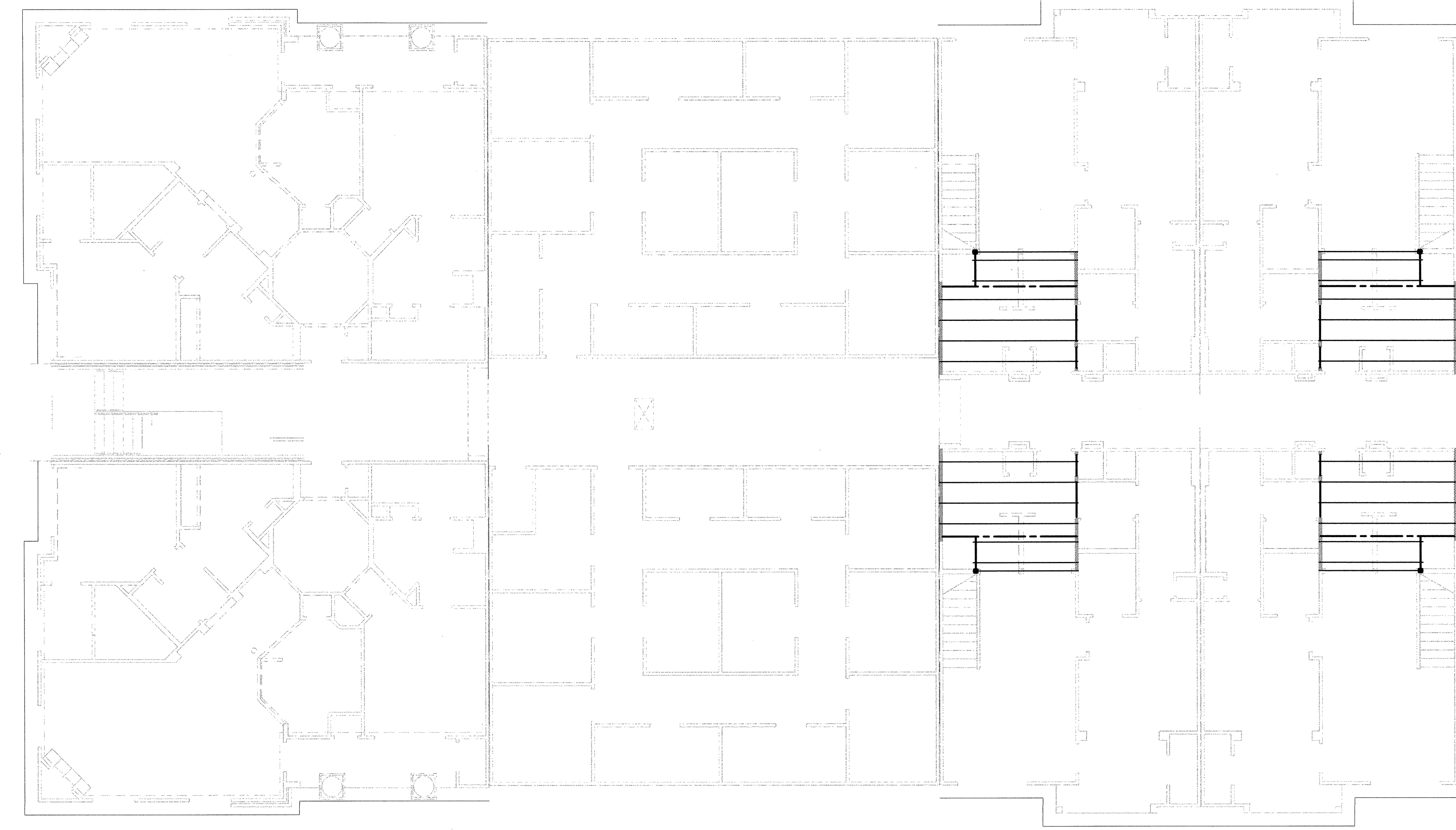
2 MEZZANINE FLOOR FRAMING PLAN - BLDG. 400B S-2.19 SCALE: 1/8"=1'-0" SEE S-2.01 FOR FLOOR FRAMING NOTES AND BEAM/HEADER SCHEDULE
